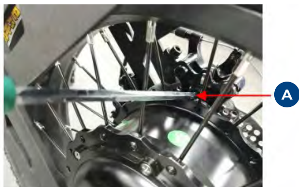
Clamping force checking
