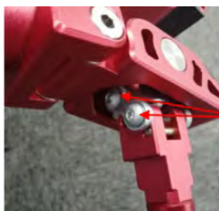
Manual clamping mechanism
