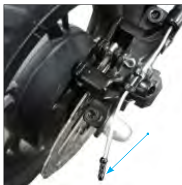
10. Put an end cable cap and use pliers to clamp tightly. At the end: Put it on a 10% slope with 120 kg load, check whether it can be parked with the brake engaged.
